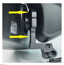
STEP 3 - Position the mount as far forward as you can. Tighten the clamp screw untill the Top and Mid Sections are slightly snug around the mirror stem.
