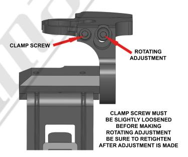
STEP 5 - Install your radar detector onto the mount. Use the adjustments shown above to adjust the RD to your desired position. We recommend adjusting the RD as close to the bottom of your mirror as you can. Be sure to tighten the vertical and pivot adjustment screws after the adjustments are made. For the Pivot adjustment, grab the long arm of the allen wrench for maximum leverage. You will not strip the threaded holes in the aircraft grade aluminum.
