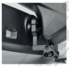
**STEP 4 -** Rotate the mount so it is parallel with the bottom of the mirror. Tighten the clamp screw untill the mount is securely attached to the mirror stem. Do not over tighten the clamp screw.
